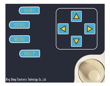
For the H2-1000KIII, use  $\uparrow$  up,  $\downarrow$  down, left or right  $\leftarrow$  to perform software operations. You can use up or down to select menu items.In addition, the instrument is equipped with an encoder, and all operations can be operated through the encoder. The encoder has three key states: left turn, right turn and Enter button (representing "confirm").
