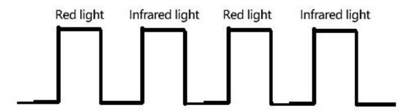
The cycle can be set by itself, but it should not be too fast. It should be controlled at about 2ms
