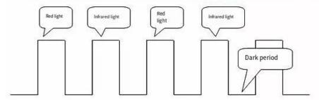
2. The timing sequence of red light and infrared light is fixed, as shown in the figure below: the luminous order of red light and infrared light can be interchanged, but the period is the same, the setting range is 200us-1ns, the dark period between red light and infrared light can be 200-1ms, and the luminous period between each group is fixed, which can be customized according to requirements, and the default can be set to 8ms.
