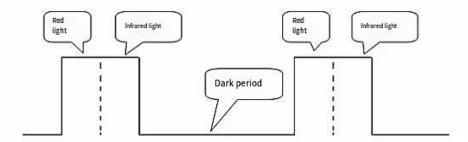
4. Red light and infrared light emit continuously with no dark interval or very small dark interval, less than 100us, as shown in the figure below
