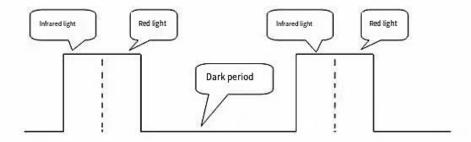
Please note: Spo2 Simulatorcan detect the first three conditions in four cases. If the blood oxygen device is the fourth luminescence driving condition, please adjust the luminescence timing to meet the three conditions. The first two driving modes are common in the market, please try your best to choose the first two driving modes.
