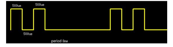
As shown in the figure above, the total period is 8ms, the red glow pulse is 500us, the infrared light emits after 500us interval, the period is also 500us, and then the rest of the cycle is all dark.
